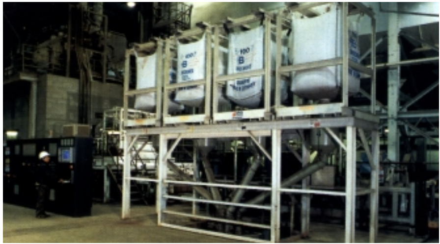
Unilock's Chicago plant has a low-maintenance granular coloring system that runs continuously for nine months a year and produces little dust.
