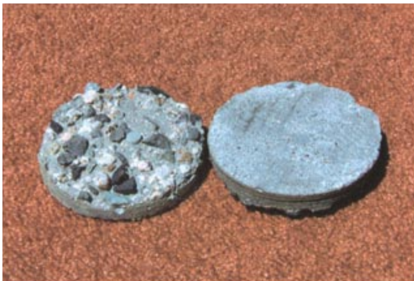
Non-metallic form ties offer a way to avoid tie hole problems since they can be cut off flush with the concrete surface. These concrete samples each contain a gray glass-fiber-reinforced plastic form tie in the center. Exposed aggregate finish on the left and smooth-ground surface on the right are from the same concrete mix.
