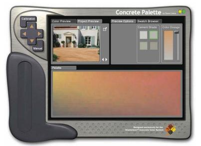
concrete producer can enter into a Chameleon<sup>™</sup> system. The Chameleon<sup>™</sup> system weighs the exact amount of primary liquid colorants according to the recipe and injects the liquids directly into the concrete mixing process.
